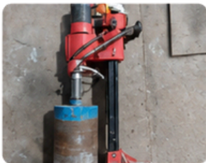
Concrete Core Drill
